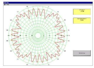
Skew Fire 4 Panels Radius 1465mm @ 680MHz Skew Fire 4 Panels Radius 1465mm @ 740MH
