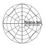
The Superturnstile is generally employed as an omnidirectional (Fig 2), or occasionally a figure eight, horizontally polarized transmitting antenna and provides excellent and reliable service in the Low, Mid and High Bands. Most frequently used as a medium power single channel antenna we also offer custom designs for two or even three channel operation. The antenna is equally suited to both analogue and digital transmissions.
