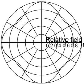
Fig. 2 Omnidirectional HRP
