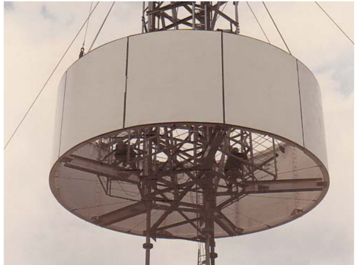
Antenna pattern testing inside a 26ft. (8m) diameter radome
