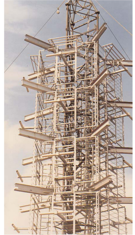
Ch.5 antenna testing at works including simulated radome supports
