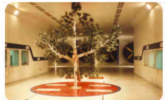
BRANCH MEMBER UNDERGOING WIND TUNNEL TESTING
