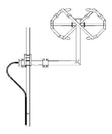
The ADB-SWB is supported by a hot dipped, galvanized steel mounting bracket for good grounding. Standard round leg mounting brackets for uniform face tower are included with each antenna, custom brackets available. Silver plated inner conductor connectors are used throughout for maximum contact life and minimum power loss.
